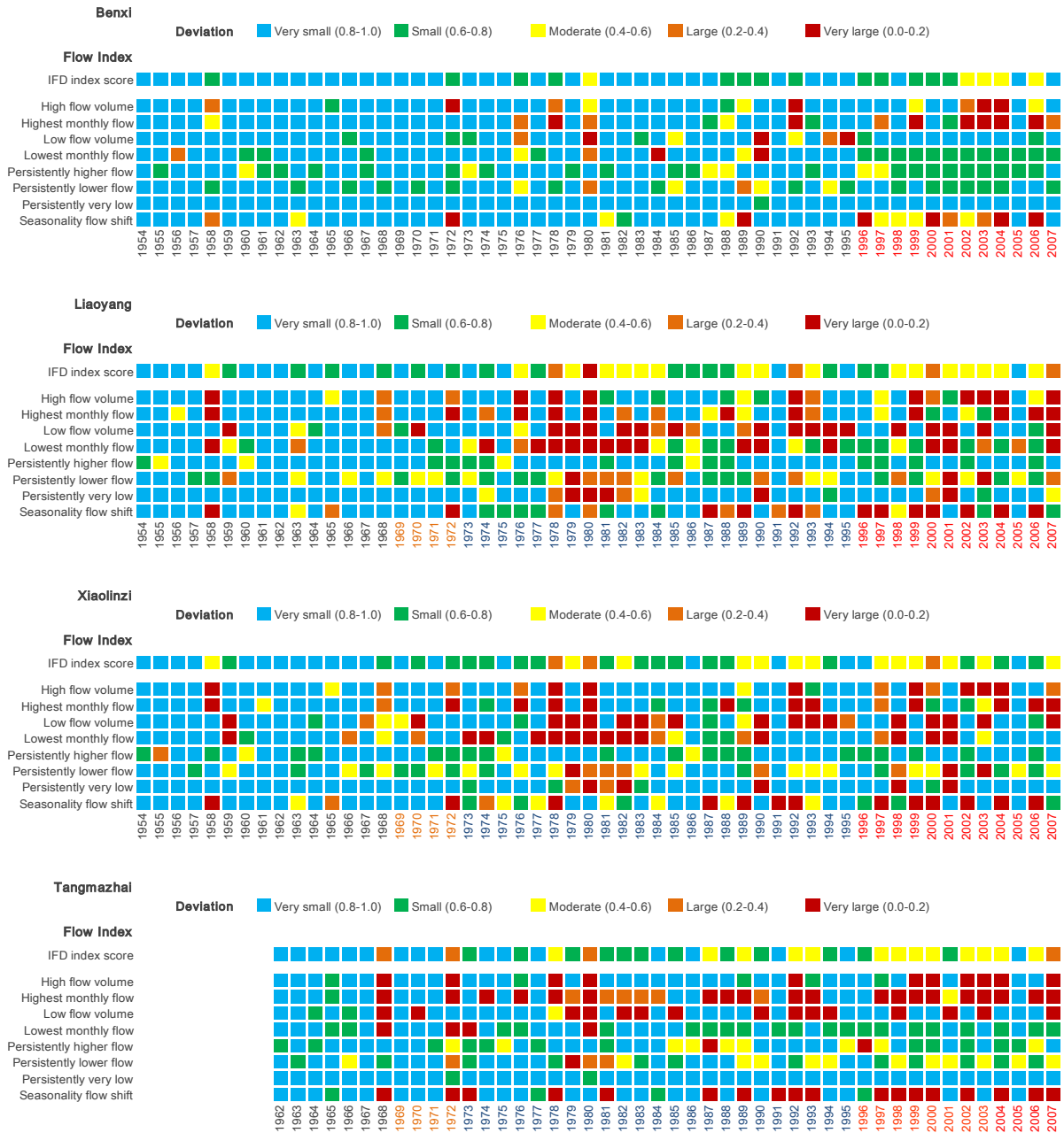
Figure 41. Time series of IFD indicator scores in 5 classes of deviation for four Taizi River stations. Coloured text for years indicates regulation phases (Table 2).
