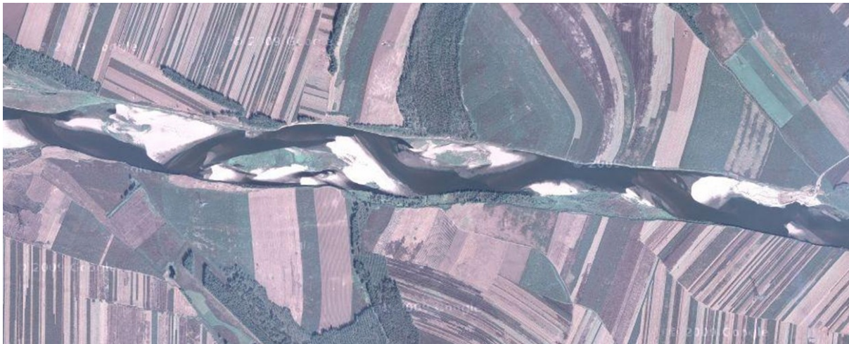
Figure 96. Taizi River downstream of Beisha River junction and just upstream of Xiaolinzi, showing alternating bar morphology. Image from Google maps.
